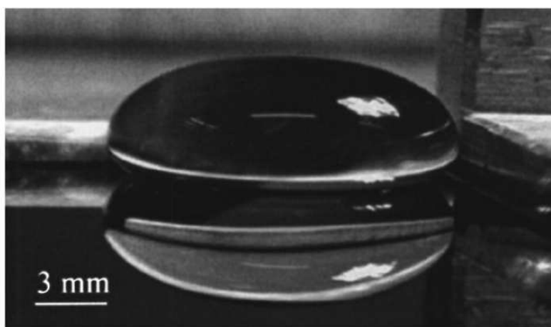
Figure 20. Leidenfrost drop; water on a heated surface. Reproduced with permission from Bianco et al. [89]. Copyright American Institute of Physics 2003.
